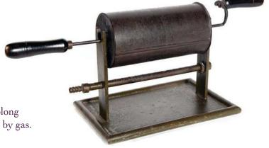
A cylindrical roaster, sheet iron, oblong model, mounted on a tray. Heating by gas. Circa 1880.
