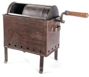
Barrel roaster, sheet iron. Suspended in a bin designed for charcoal.
