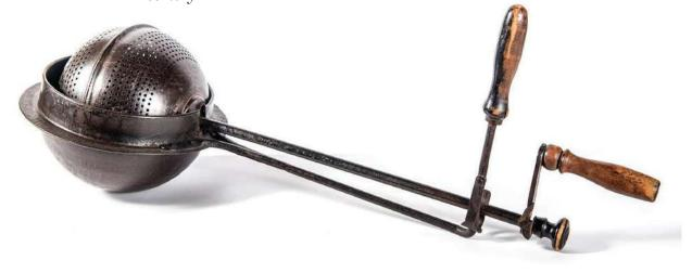
Spherical roaster, sheet iron, connected with a spirit burner. Germany, 19th century.
