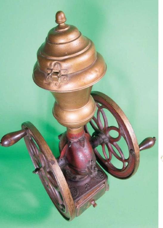
Counter mill with two wheels, cast iron with brass-colored closed hopper, 19th century.
